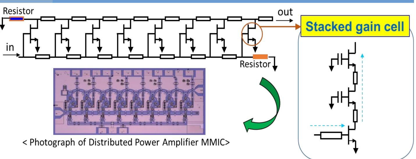
Designing Power Enhancement Using Stack Structure
