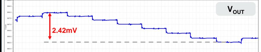
Fig.3 Post simulated steady-state waveform of  $V_{OUT}$  ( $V_{REF} = 0.95V$ )
