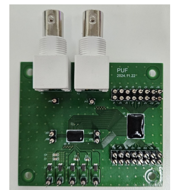
Fig. 6. Layout of PUF operating circuit (left side) and PCB of PUF operating circuit (right side)
